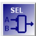
The **Analog selector block (SEL)** allows an digital value to select one of two analog input values.
