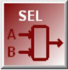
The **Digital selector block** (SEL) allows an digital value to select one of two digital input values.
