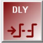
**Delay (DLY )** function blocks will introduce a specific fixed delay when triggered. The delay time is adjustable.
