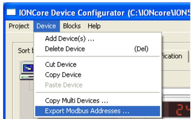
This will create a text file containing all the defined Modbus register addresses for the selected device, a sample is shown below:
